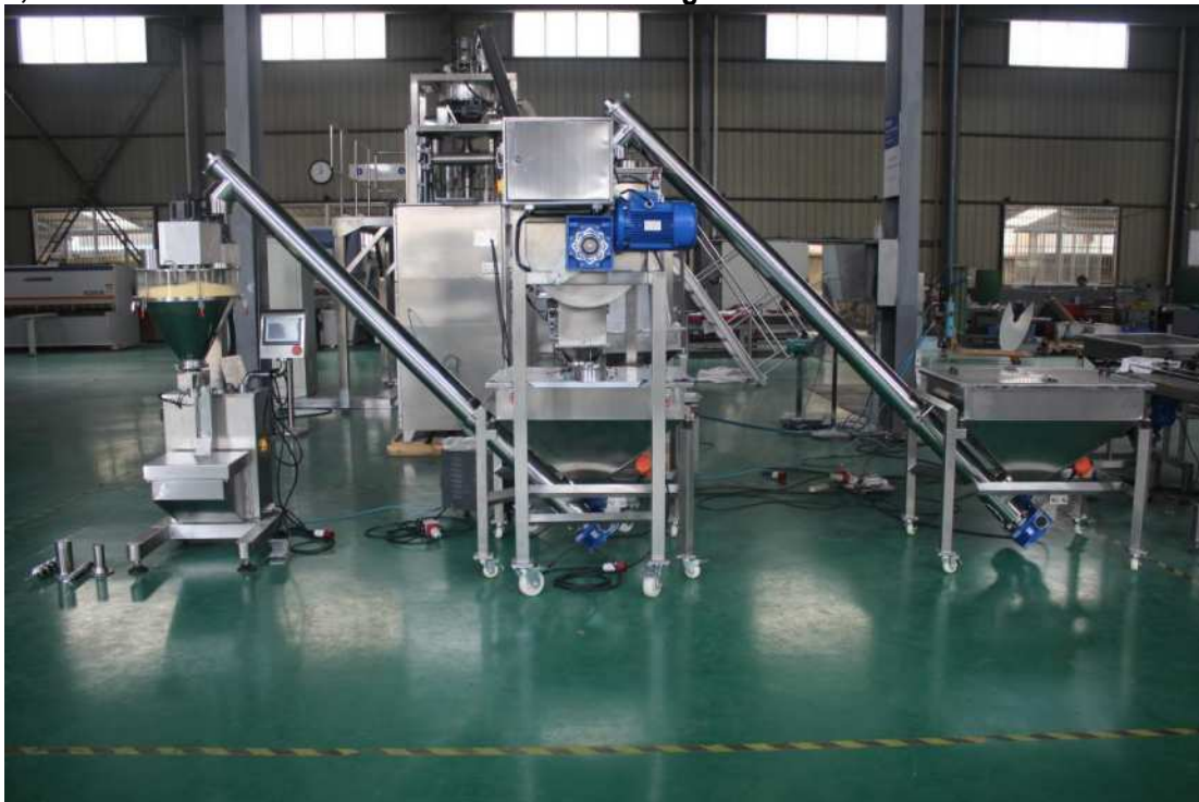
4, screw feeder + ribbon mixer + screw feeder + auger filler
