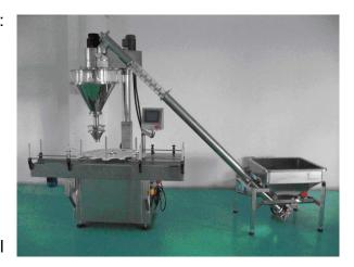
Screw feeder working with vertical packing machine:
