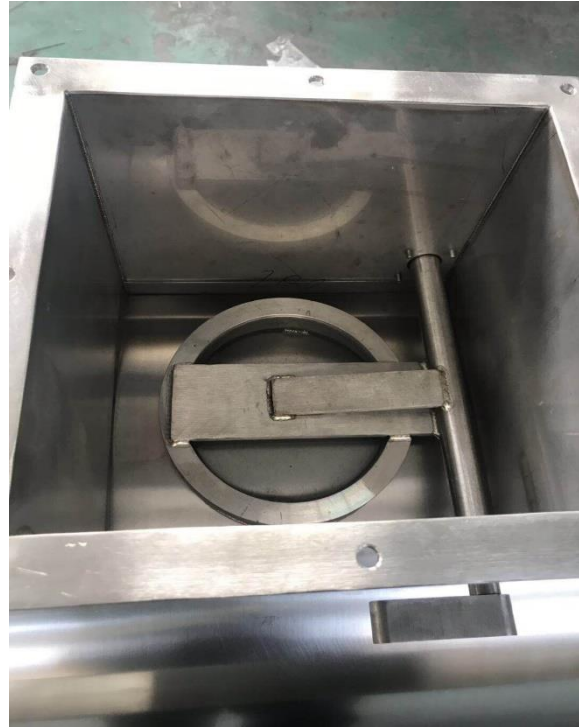
The discharge port from the outside of the mixer
