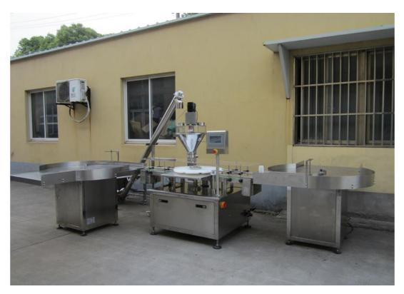
This series could do work of measuring, can holding, filling, weight chosen. It can constitute the whole set can filling work line with other related machines, and suitable for filling kohl, glitter powder, pepper, cayenne pepper, milk powder, rice flour, albumen powder, soy milk powder, coffee powder, medicine powder, essence and spice, etc.
