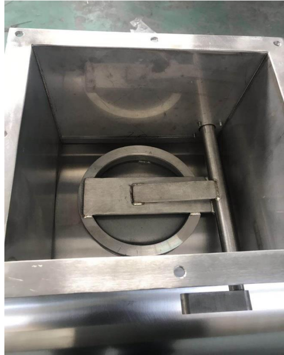
The discharge port from the outside of the mixer
